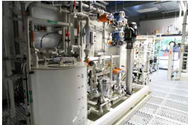
Demineralized water production from ultrafiltrate
