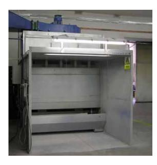
Paint coating with the use of water screen or dry separation depending on desired performance and amount of oversprays
