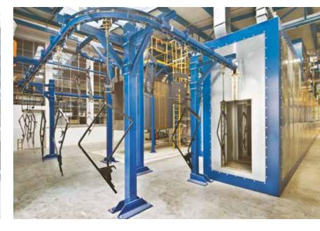
Equipment for manual and automatic paint coating
